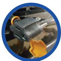
Auxiliary 110V power receptacle (125K thru 400K)
